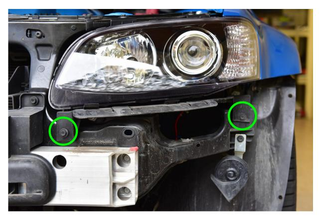
$\label{eq:Step3} \textbf{Step 3}$  Remove the two bolts securing the bottom headlight brackets.
