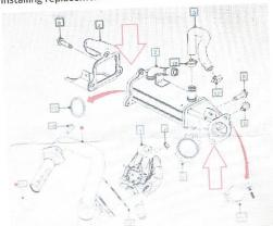
Step 4: Utilizing the supplied coolant hose/hose barbs/hose clamps, join the two coolant hoses that are connected to EGR cooler. This will require cutting the hoses in positions indicated. Pre-measure and check before cutting to ensure hose will have sufficient length and not contact any other components.
