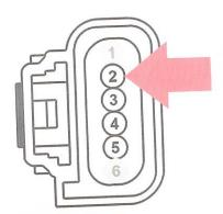
Step 6: Disconnect vehicle battery. Disconnect MAF sensor (sensor on air filter box), remove a few inches of plastic wiring protection and cut circuit 2 wire. Solder the supplied resistor in line with circuit 2 (resistor orientation does not matter). Insulate the new connections and refit wiring. Note, on most models circuit 2 is the BLUE wire. The circuit locations are numbered on the back of the connector. (Picture is a front view of the connector).
