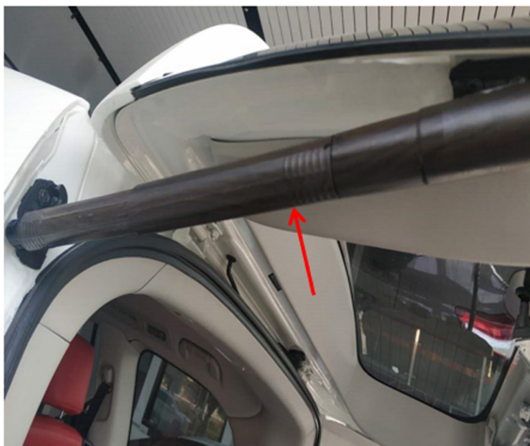
4: Install the ball and socket of the special electric brace in the direction of the brace line and install it on the door bracket (left and right are the same)
