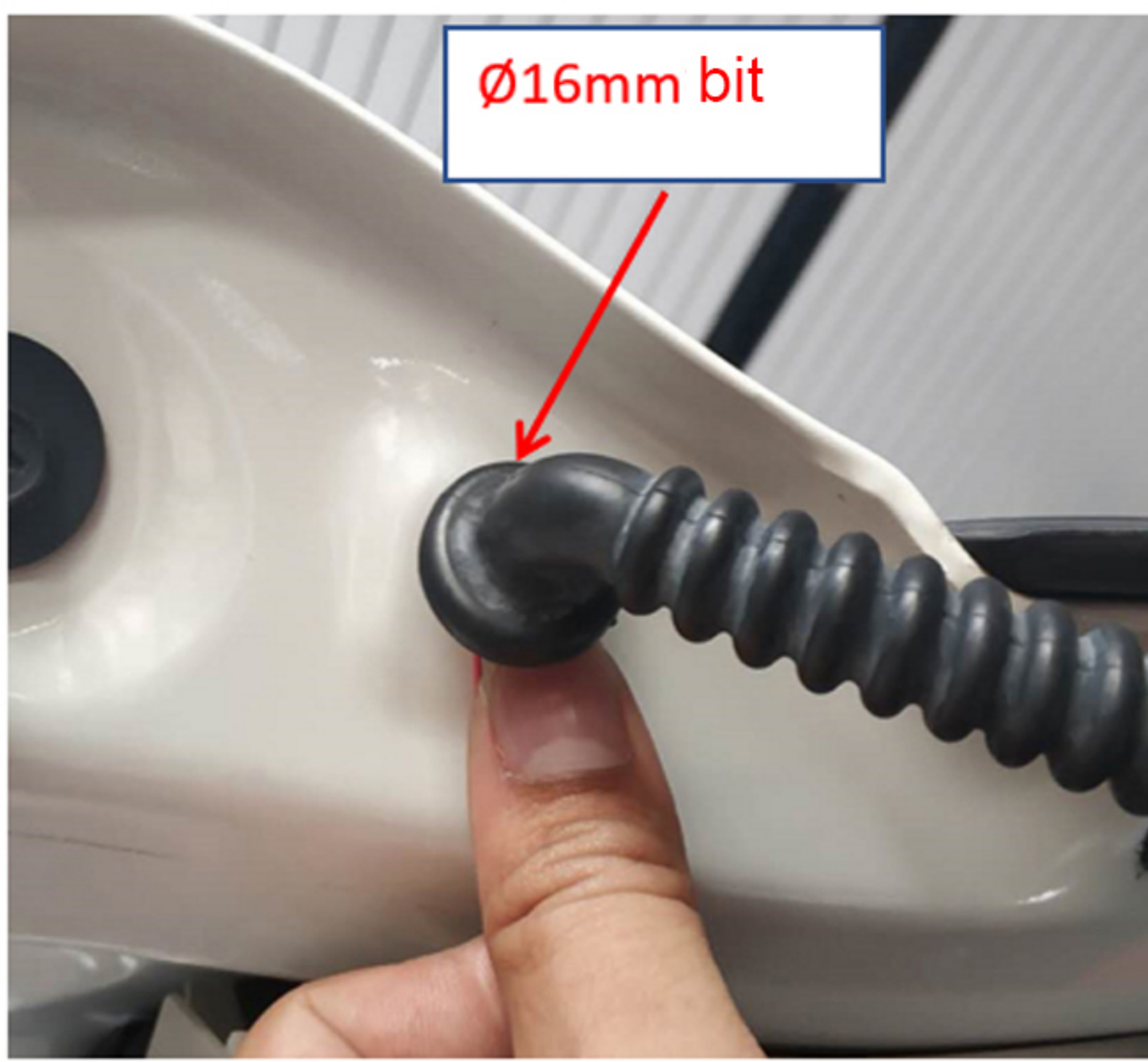
6: Use a 16mm drill bit to drill holes above the stay bar to pass through the motor wire, and plug the corrugated pipe rubber plug
