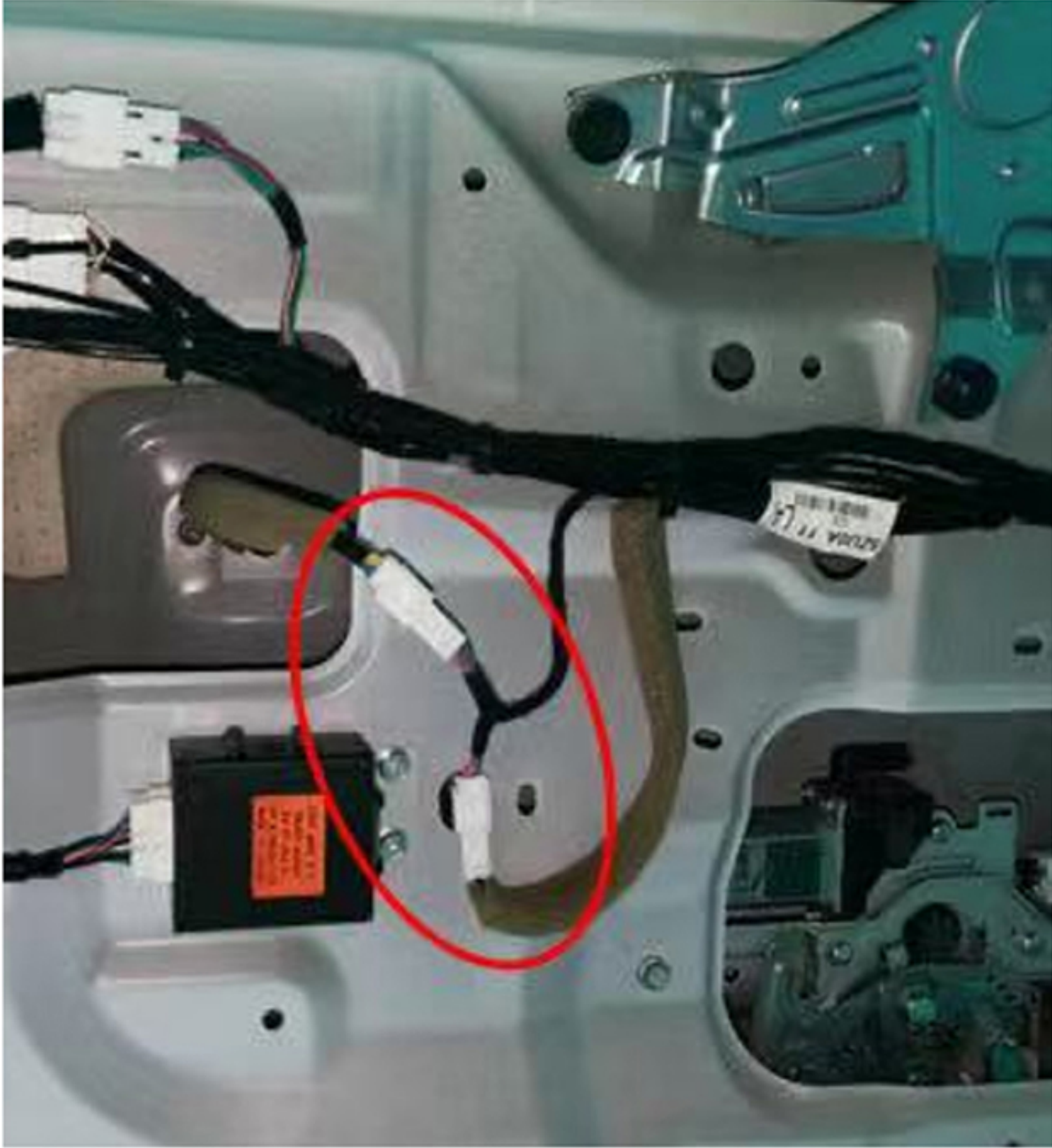
10: The tailgate key plug on the lock cable is connected to a pair of plugs
