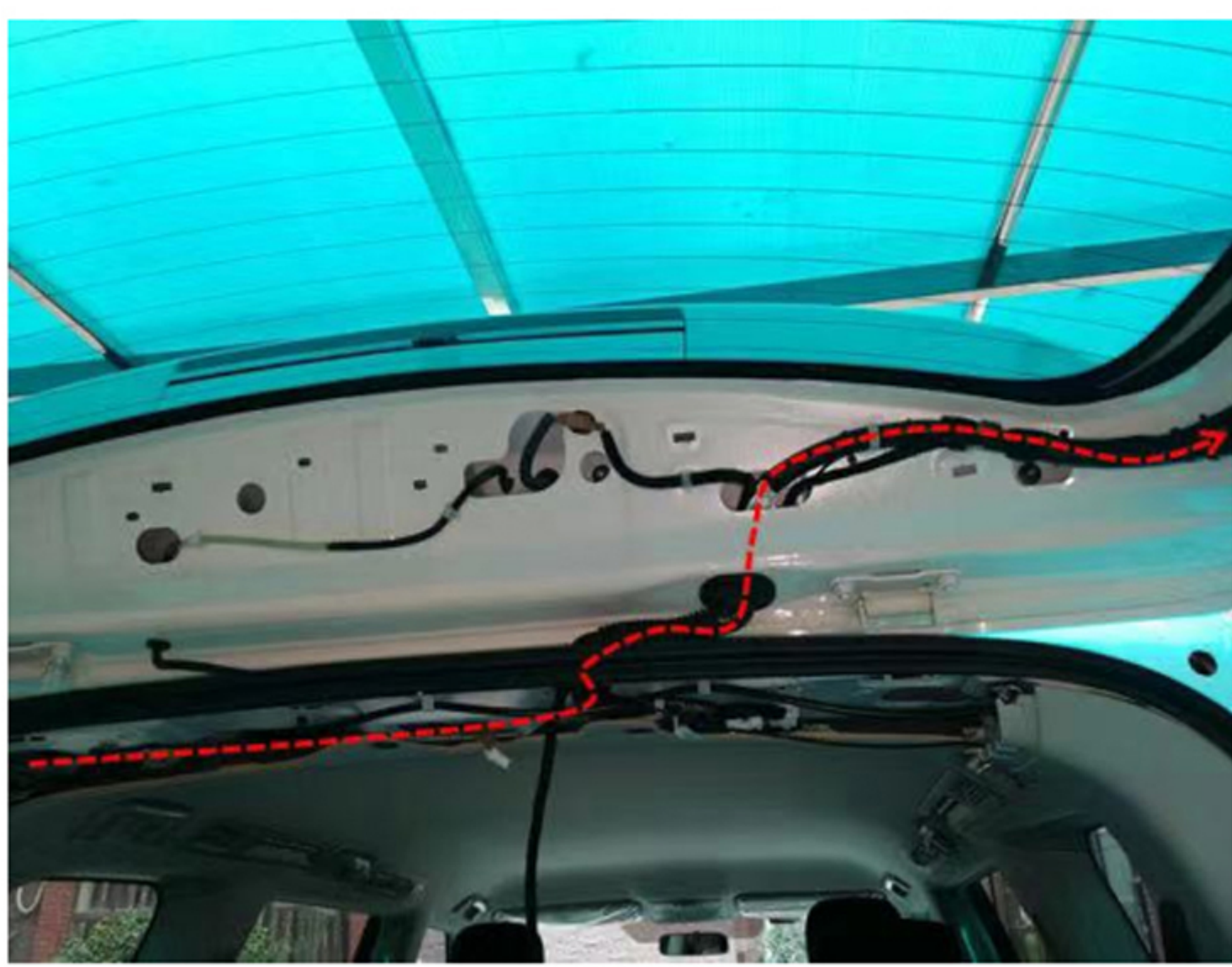
8: Pass the power cord/front key cord/CAN cord through the bellows of the original vehicle from top to bottom
