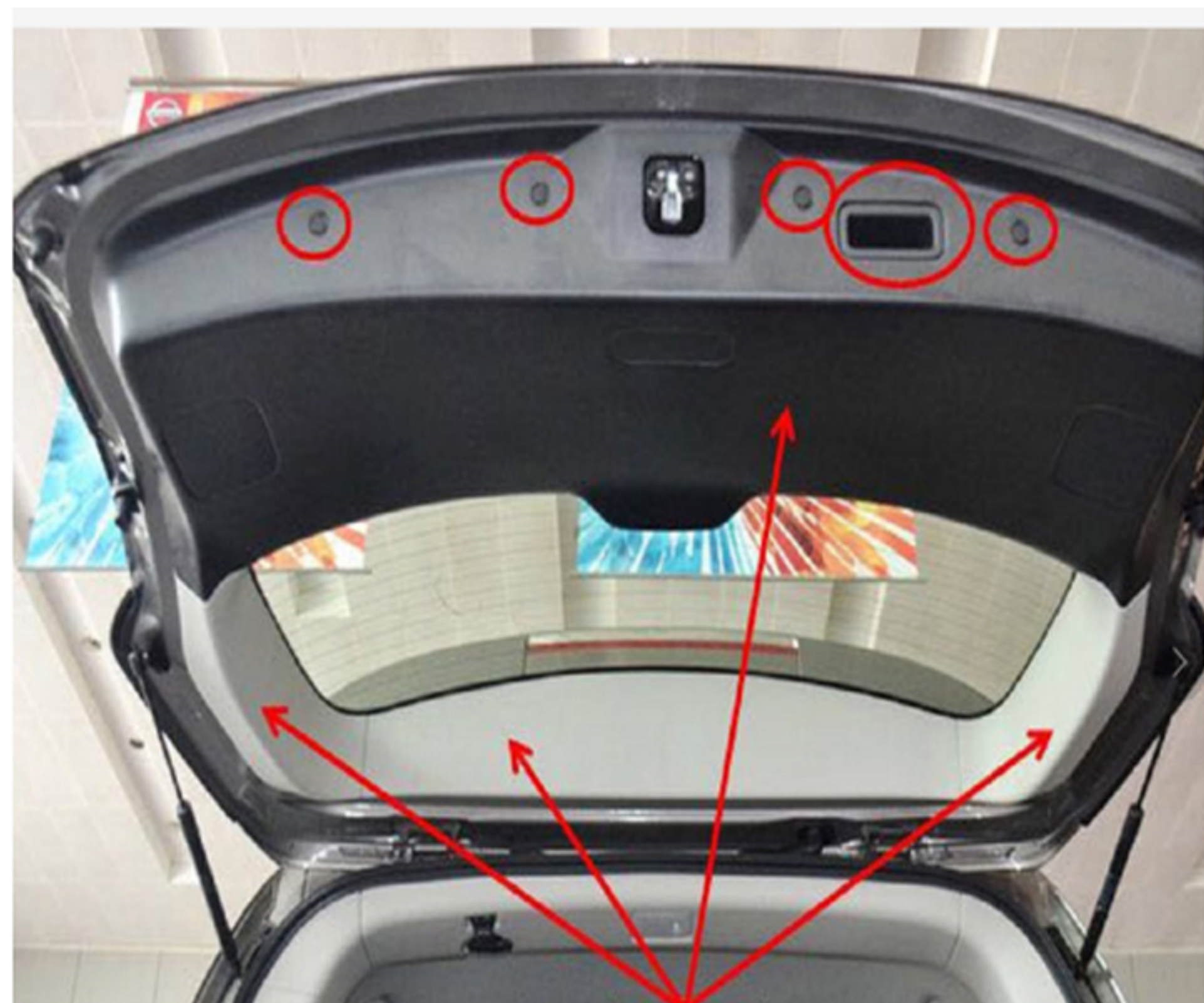
3: Remove the original door bracket and install the special door bracket. Note that the direction arrow of the bracket points to the tail lamp, which is left and R is right (both sides are the same)
