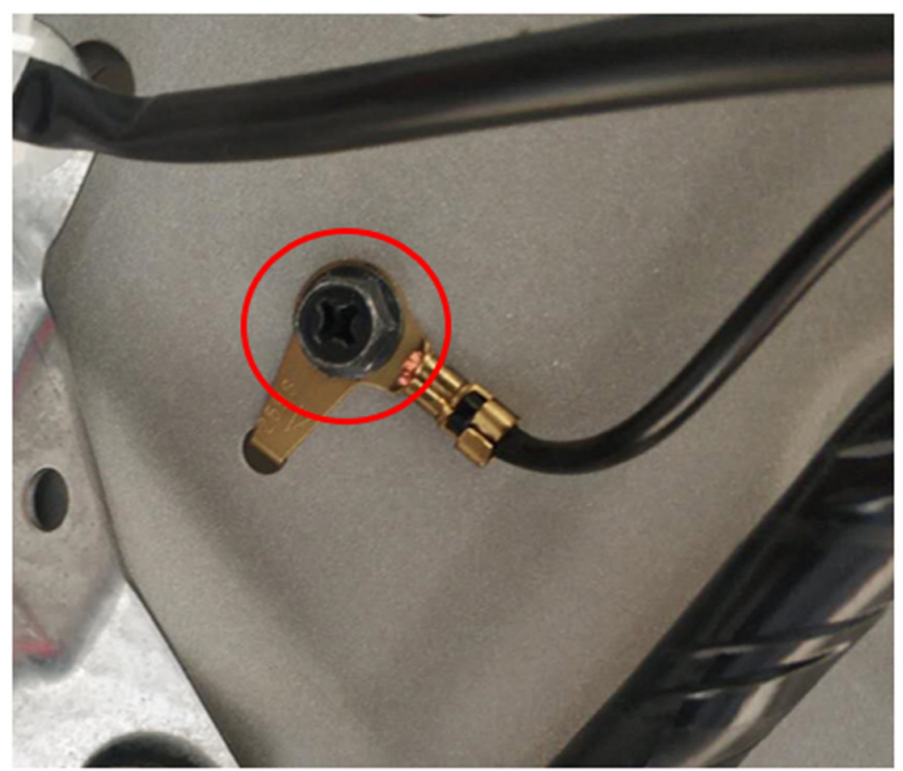
9: Connect the ground wire to the tailgate ground
