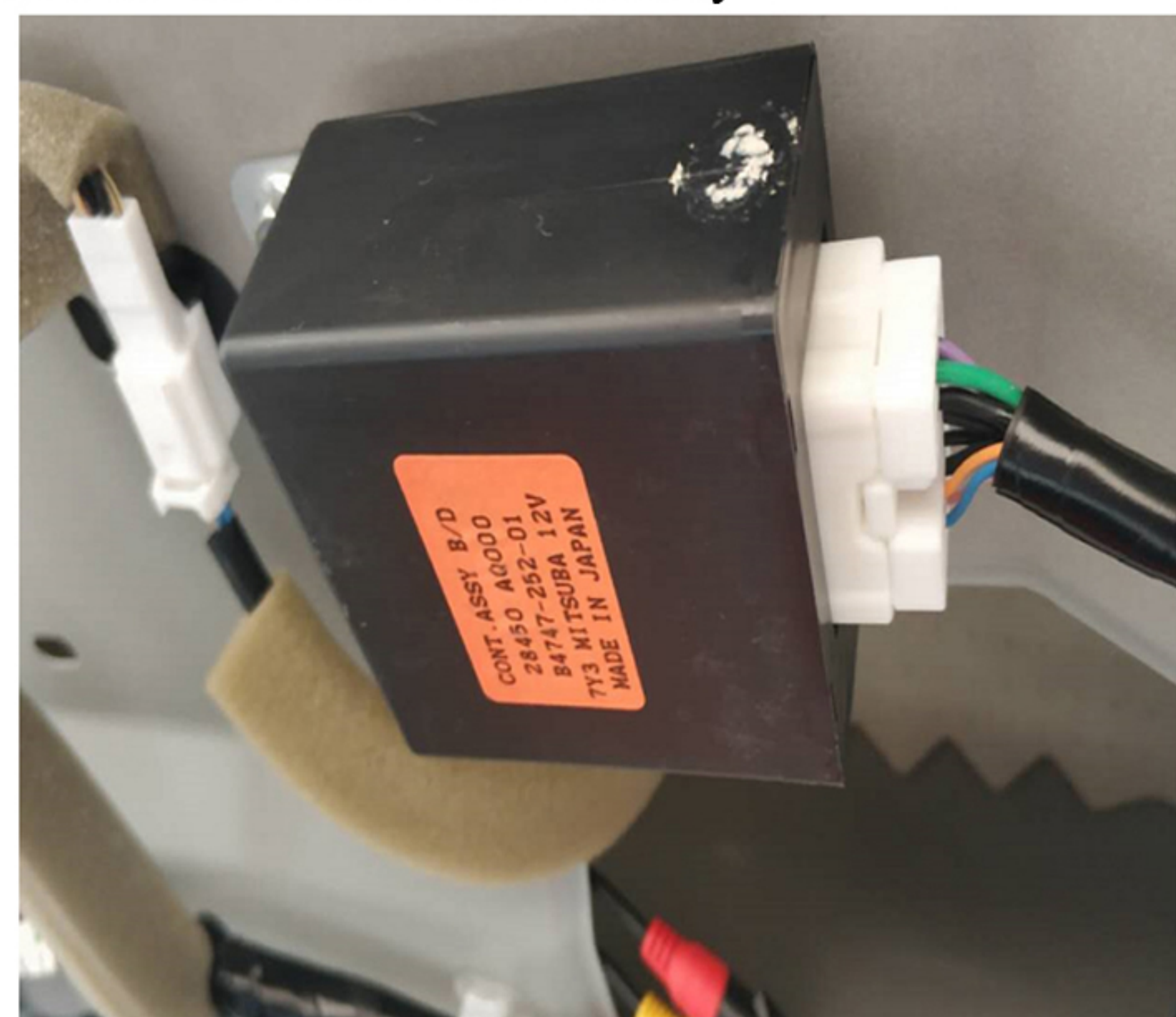
18: After the tailgate is installed, pull out the plug for 1 minute and then plug it back. Note: This operation must be performed when the ECU of our company is powered on, otherwise the electric suction lock of the original vehicle cannot work normally
