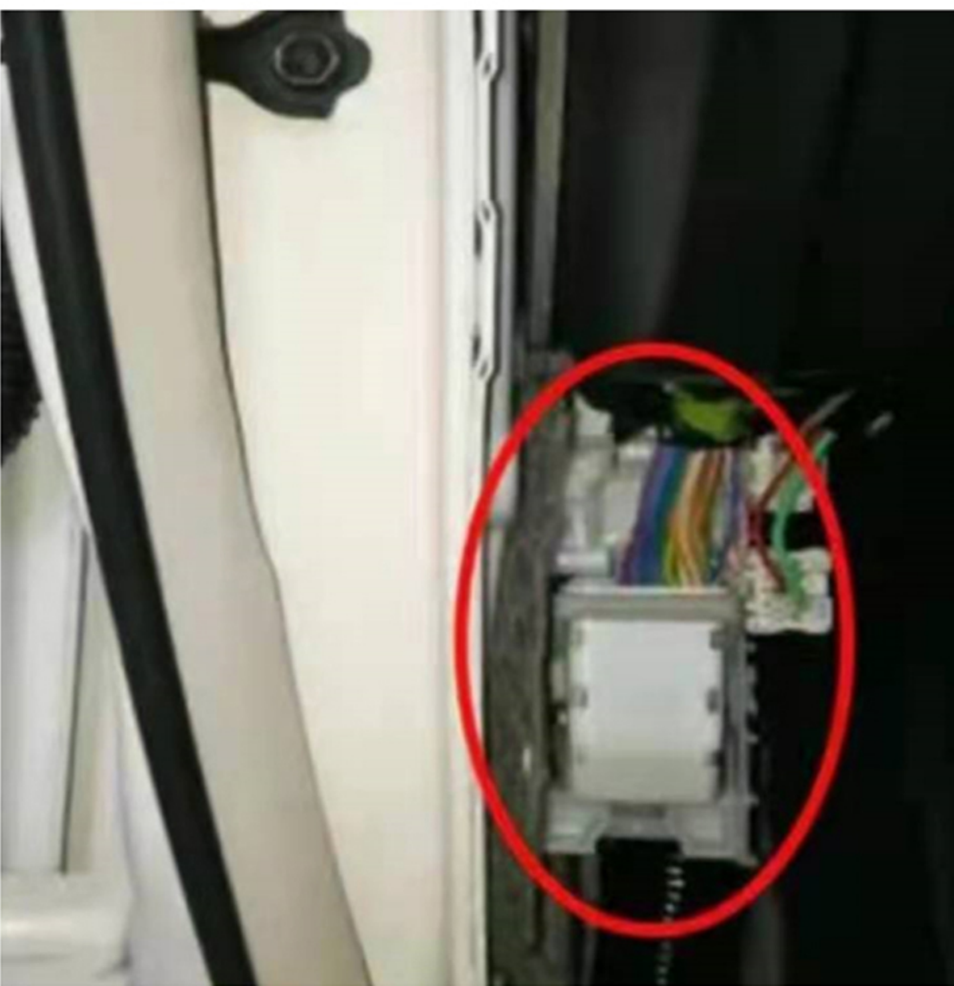
12: The CAN line is on the large white plug in the left triangle
