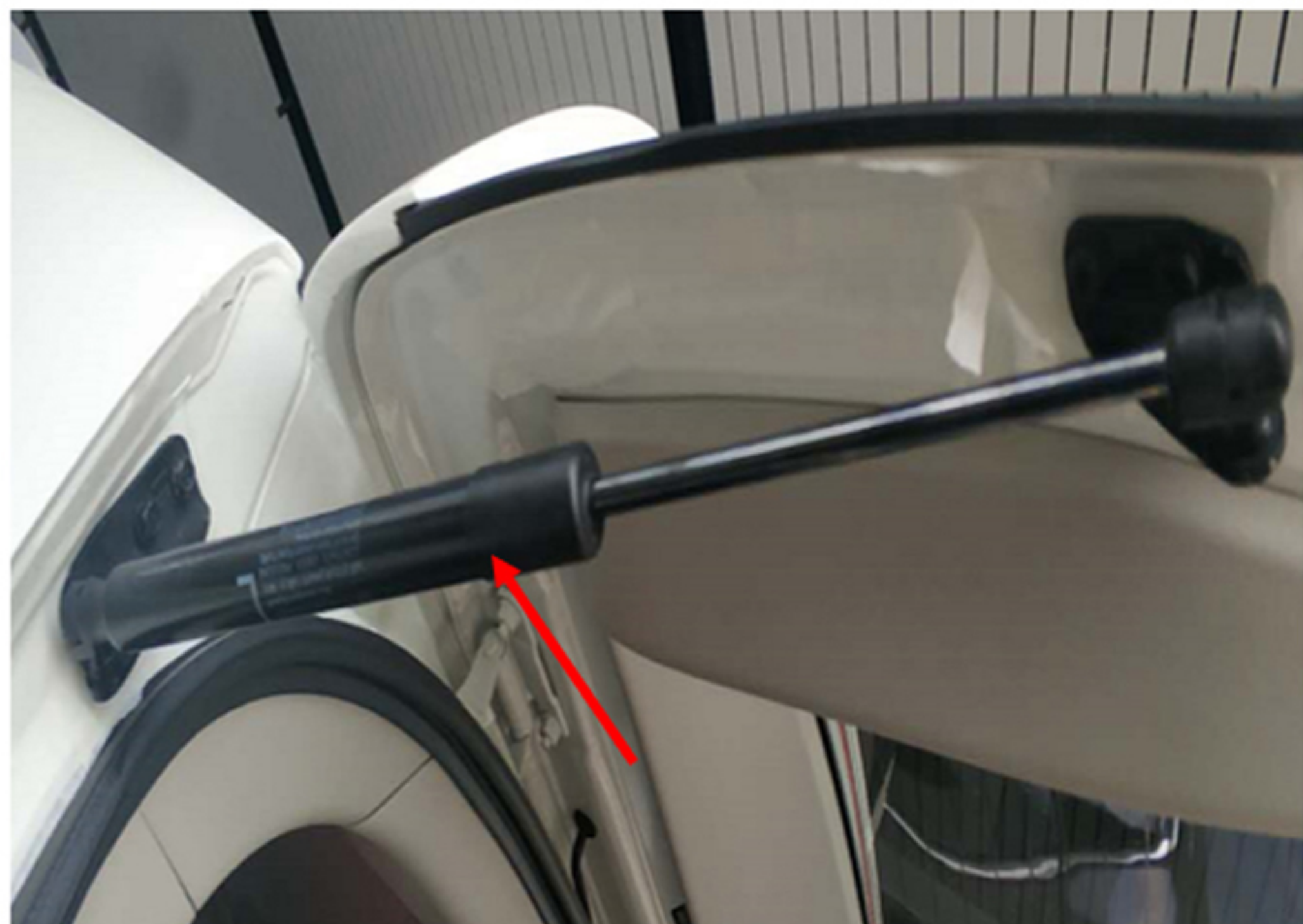
1: Remove the original air strut (left and right are the same)
