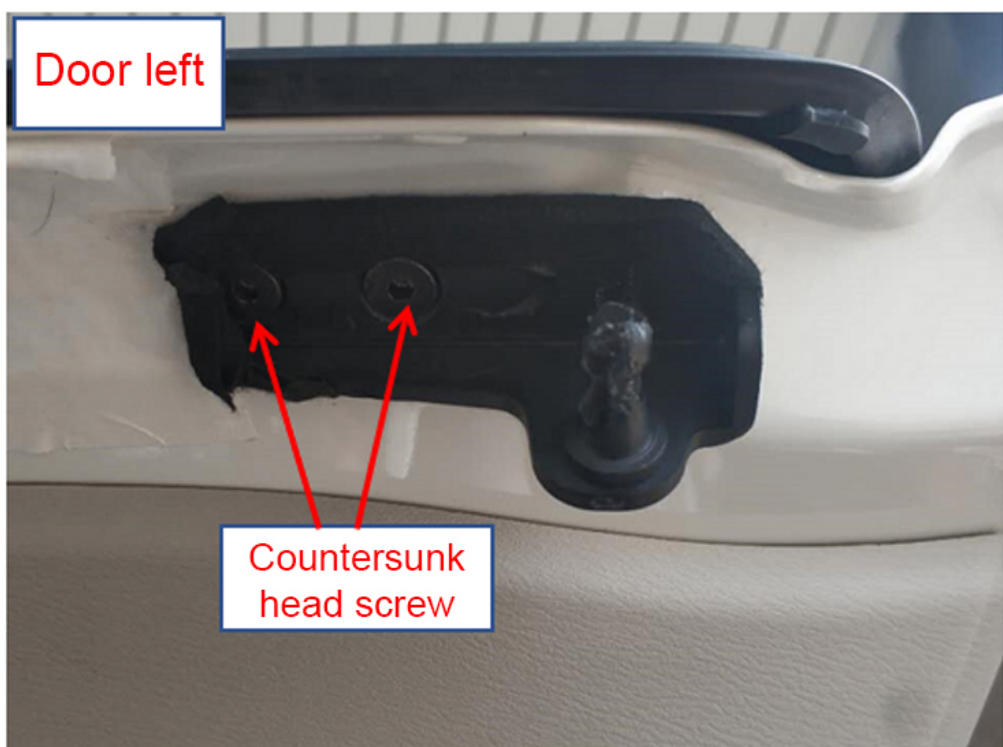
3: Remove the original door bracket and install the special door bracket. Note that the direction arrow of the bracket points to the tail lamp, which is left and R is right (both sides are the same)
