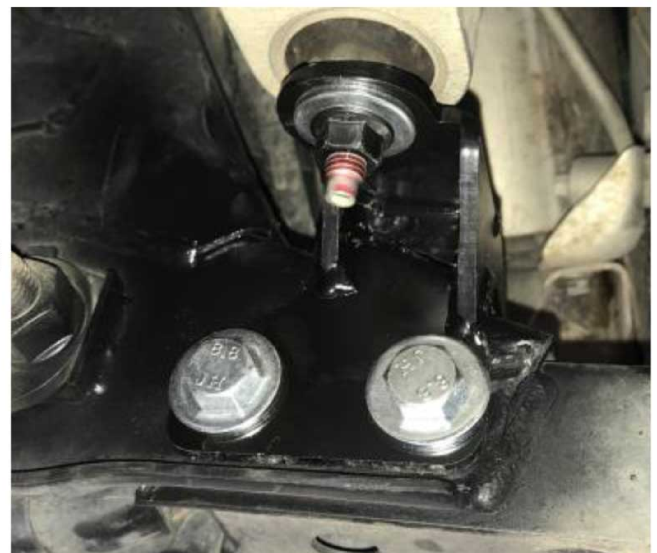
FIG 4&5. Fit bracket as shown in images using the 2 x M10x1.50P x 110mm long bolts with M10 Flange nuts and washers supplied. Reinstall factory bolt through diff mount into new bracket, fit supplied washer and flange nut, leave loose until the end of installation procedure.
