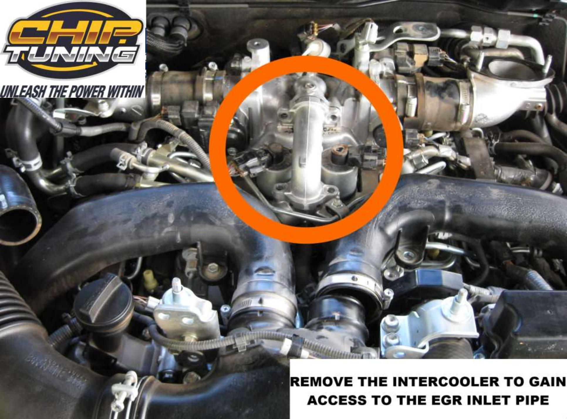
**REMOVE THE INTERCOOLER TO GAIN
